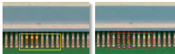
Lifted leads clearly identified using angle view camera.
