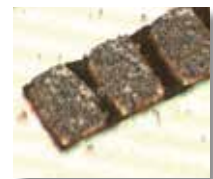
2D+3D Image with clear low bridge defect
