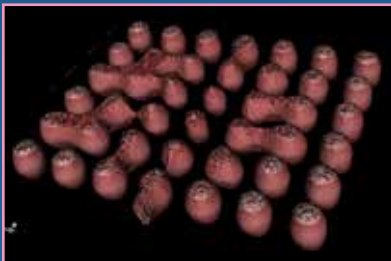
BGA short / open 3D CT Inspection
