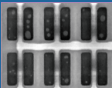
Void Inspection of LED
